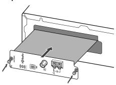
When the board meets the internal connector, apply a little more pressure so that the board plugs fully into the connector. Make sure the board's panel is flush with the T-4555P's rear panel.
